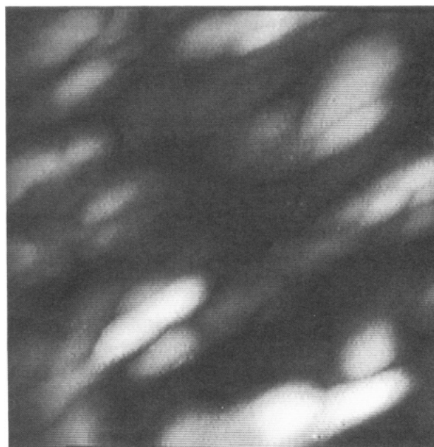
Figure 1. STM image of a gold film grown by CVD on a glass substrate. The image is obtained using a Pt/Ir tip with a bias of 1.00 V and a tunneling current of 2.0 nA. The image is 400 × 400 Å and the vertical scale is 40 Å from darkest to lightest.
